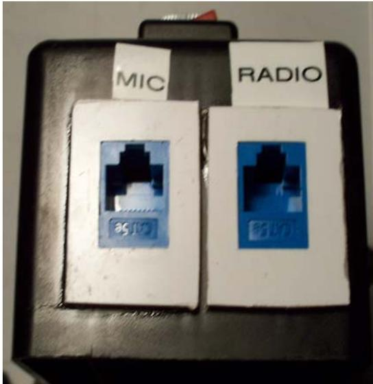
8 Pin modular connector to radio and Mic
